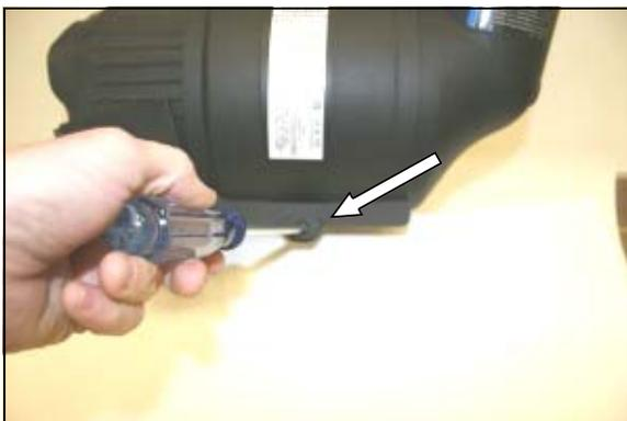
**1.** Loosen the screw that holds the inspection cover on the top of the factory air box.
