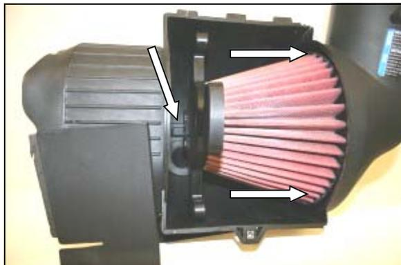
6. Carefully align the notch on the Airaid Premium Filter with the raised rectangle at the bottom of the factory airbox, then slide the air filter towards the elbow. Make sure the air filter is seated inside the factory housing securely. Next, replace the factory inspection cover, and tighten the screw.
