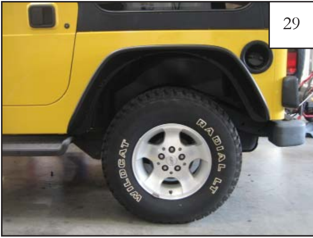
Completed rear driver's side flare installation.
