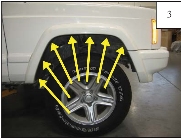
Using a 10mm socket & wrench, remove the remaining factory fasteners on the factory front flare (7 locations). After all fasteners are removed, pull firmly to remove factory flare.
