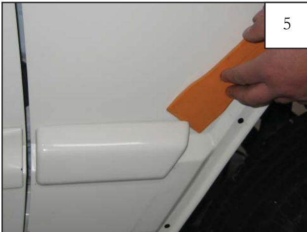
(For 97-01 Model Years Only) Remove body side molding on front fender using a putty knife or plastic type remover, taking caution not to scratch the paint. Save molding for optional trimming and reinstallation.
