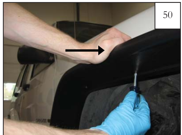
Hold flare in place on fender and start a #8 pan head screw into each hole location and through speed clip on inner structure (6 places). Do not fully tighten.
