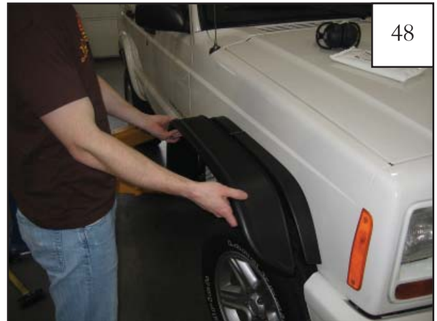
Place the outer flare over the inner pieces and push until snug against the sheet metal. Make sure the inner splash shield is tucked behind flare.
