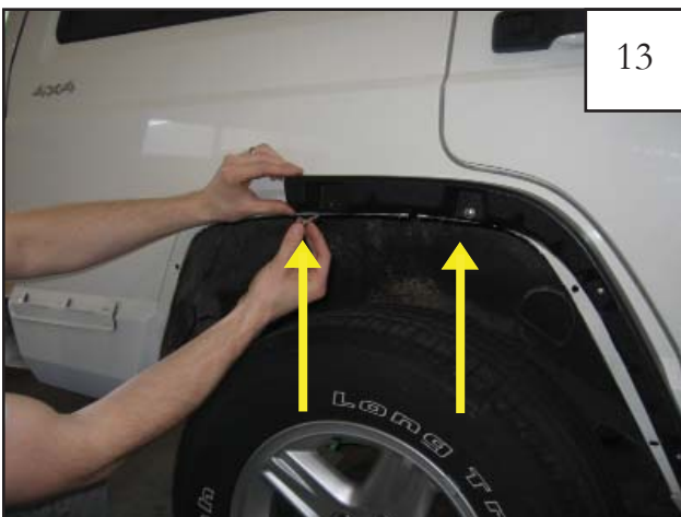
Position inner piece P3 (D3 for driver side) on fender, aligning top two holes in the inner piece with existing factory holes in sheet metal. Slide washer onto M5-.8 machine screw. Insert a screw/washer assembly through inner flare piece and fender and secure with a flange nut. Only hand tighten at this time.
