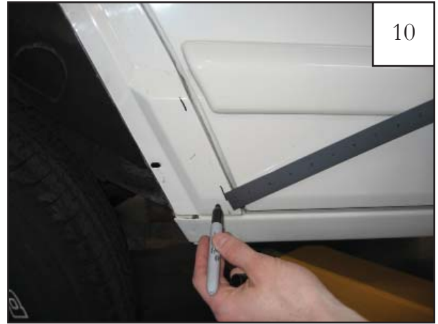
(For 4-Door Vehicles Only) Use a grease pencil or removable marker to make a line parallel with the door seam \frac{3}{8} " away from the door seam.
