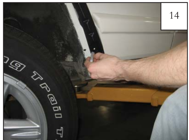
Align outer edge of inner piece P3 (D3 for driver side) with the measuring lines made in Step 10/11. Use a grease pencil or marker to mark the lower front hole location on the sheet metal.
