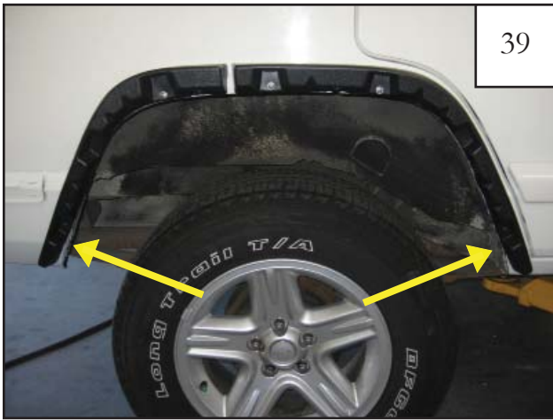
Install tuflocks in two lowest hole locations on inner pieces P3 & P4 (D3 & D4 for driver's side).
