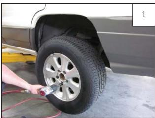
Remove tire using an impact wrench.
