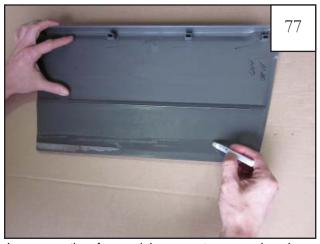
In preparation for applying new tape, apply primer using supplied primer applicator (AD1-0006) to plastic along bottom edge of side cladding.
