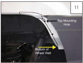
Make line extending from the bottom of the wheel well to approximately 1-1/2" above the top mounting hole. The line should be 1/4" in from edge of the wheel well.
