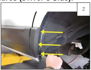
Using a #2 Phillips Screwdriver, remove factory screws from upper side cladding (3 places). Remove cladding.
