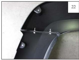
Using a 7/16" wrench and 3/8" socket, bolt rear main flare to bumper piece using supplied screws (SW1-0006) and nuts (NU1-0011). Do not fully tighten screws. Parts are marked on the inside. Driver's side: D3 for main flare, D4 for bumper piece.
