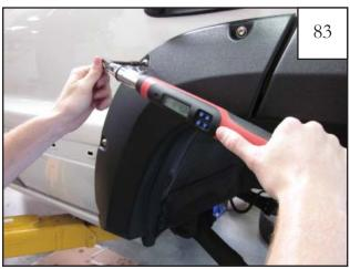
Once all screws have been started, snug screws to vehicle. Torque screws to 24 in•lb (2 ft•lb). **DO NOT OVERTIGHTEN!**
