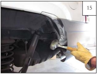
Using a hammer, pound the tabs made in the inner sheet metal flat against wheel well.
