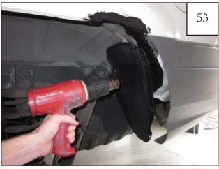
Using a heat gun, heat splash shield until pliable and use heavy work gloves to push and mold splash shield into place aligning with inner wheel well. Hold in place and allow to cool. Then fully install push retainers into splash shield.
