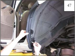
Hold cut cover in place and mark inner wheel well through holes in part (4 locations).
