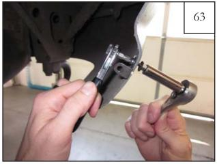
Using a Phillips screwdriver and a 3/8" socket wrench, tighten the nut and screw together. NOTE: Some adjustments may need to be made to the bracket for proper flare positioning. Once brackets have been adjusted properly, fully tighten.
