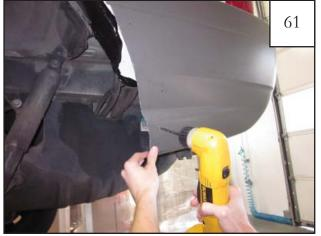
Using a 3/16" drill bit, drill the two holes marked in step 60.
