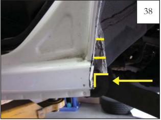
Cut away lower corner of pinch weld.
