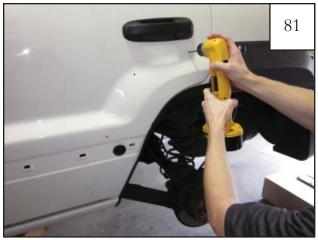
Using a 3/16" drill bit, drill holes marked in step 80.
