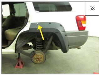
Install one screw (SW1-0045) in top front hole of flare to hold it in place while making marks in the next step.
