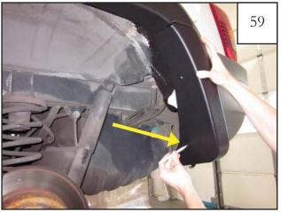
Hold flare and bumper piece in place so that the holes in the bumper piece barely overlap the cut bumper and mark the locations on the edge of the bumper. Use an awl if needed (2 locations).
