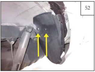
Re-install splash shield using supplied panel retainers (RV1-P008). *NOTE: Do not fully install push retainers. Splash shield must be re-molded.* See step 53.
