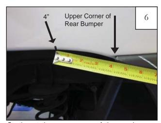
Starting at the upper corner of the rear bumper, measure forward 4" along upper edge of fender lip and make a mark extending up 1/4".
