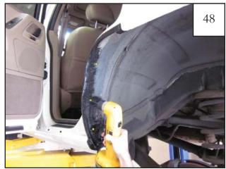
Remove part and drill marked locations using a 3/32" drill bit (4 locations).
