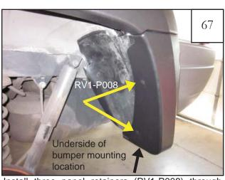
Install three panel retainers (RV1-P008) through flare and into mounting brackets and underside of bumper mounting location as shown.
