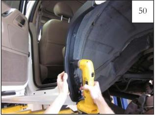
Place cover piece back on vehicle. Using a #2 phillips head, install screws (SW1-0056) through cover piece into holes drilled in step 100. Remove excess caulking along edges if needed.
