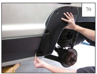
Close rear door. Hold door piece in place on door aligning it with rear main flare and trace outer edge of flare onto cladding
