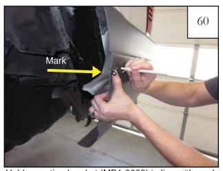
Hold mounting bracket (MB1-0003) in line with mark made in step 59 and make a mark through the hole location in the bracket. Repeat for second bracket.
