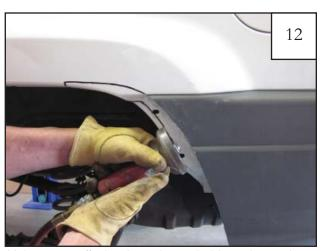
Using a cut off wheel or other suitable tool, cut along line marked in step 11 removing the inner flange.
