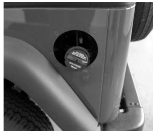
Figure #1 – Remove Gas Tank Outer Flange
