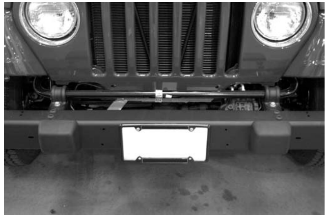
Figure #8 – Factory Front Panel Removed
