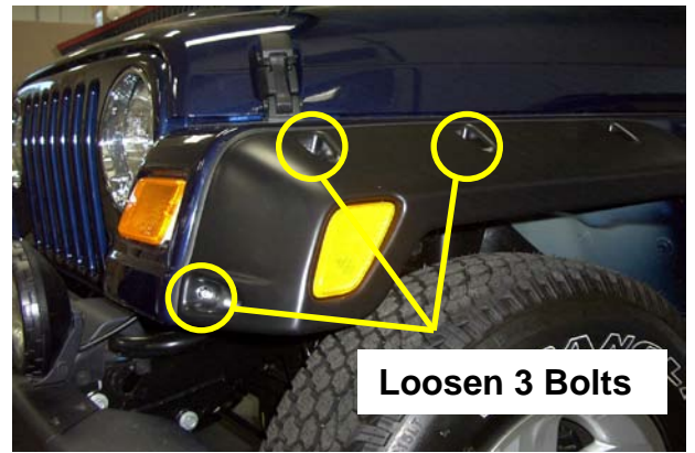
Photo #2 – Loosen Bolts (Do NOT Remove)
