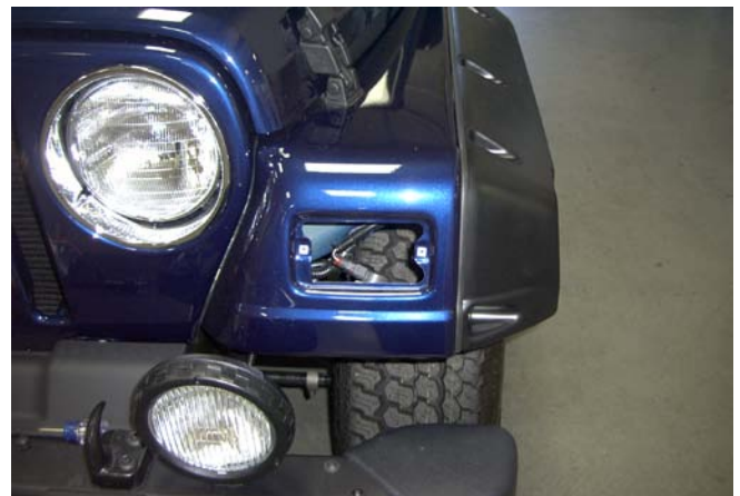
Photo #1 – Front Marker Light Cover Removed
