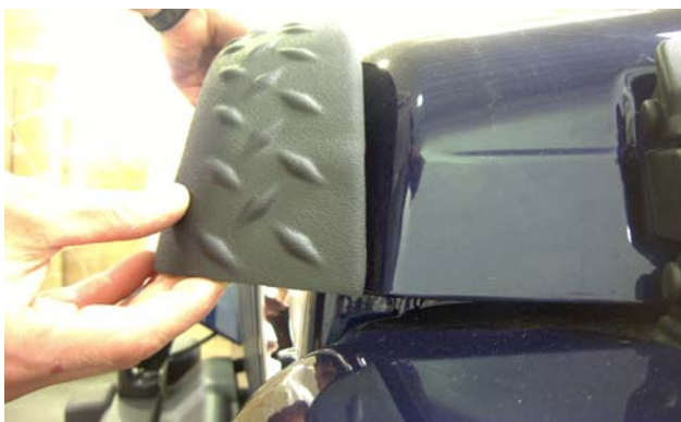
Photo #5 – Hood Protector placement
