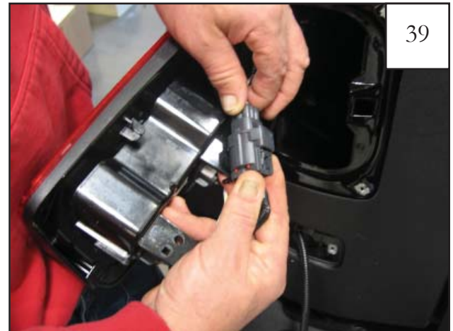
Reconnect light connector of tail light.
