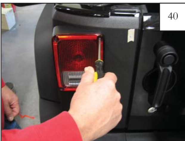
Using a #2 Phillips screwdriver, reinstall tail light.
