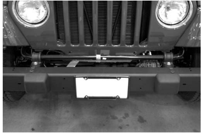
Figure #8 – Factory Front Panel Removed
