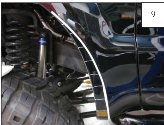
Mark fender with grease pencil about every 2" up to edge of masking tape.
