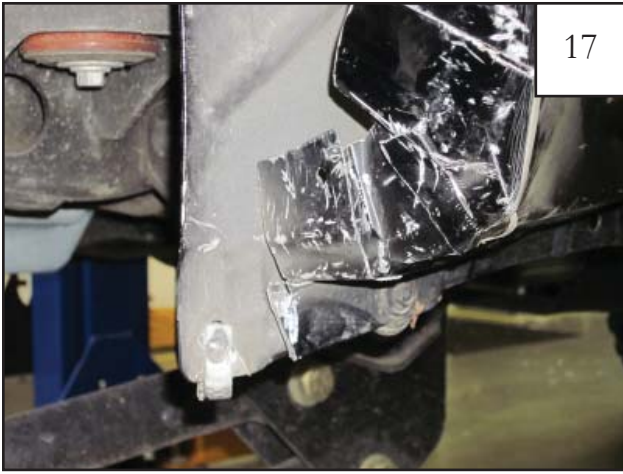
This is how it should look after you cut off back lower flange.
