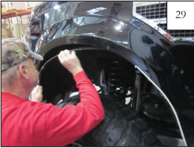
Reinstall splash guard using saved factory clips to fasten to outer edge.
