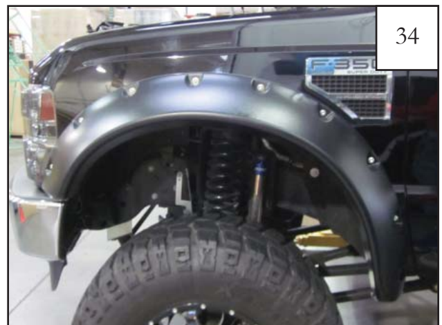
Completed front flare installation.
