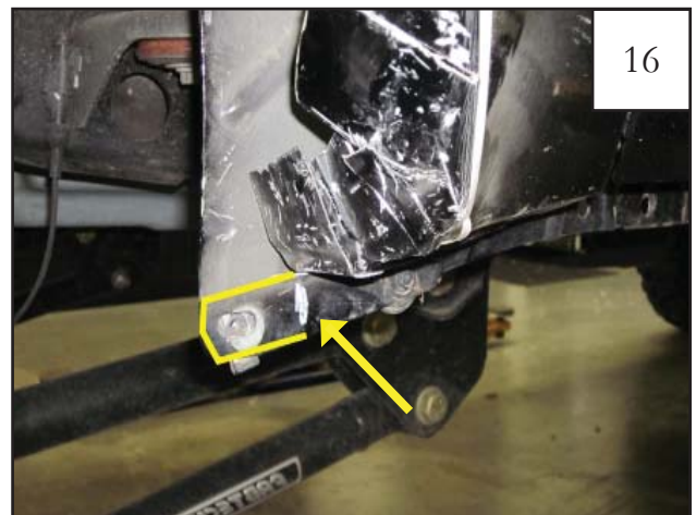
Using a grease pencil, make a line on flange at back of wheel well parallel to the outer edge. Using a cut-off wheel, cut away flange area indicated. DO NOT CUT BACK WALL OF WHEEL WELL. See step 17.
