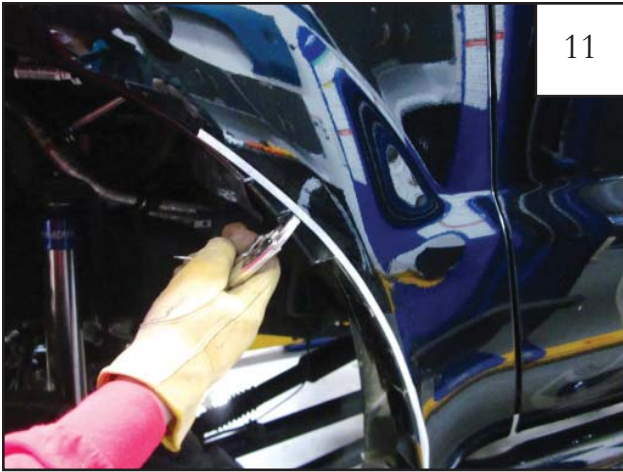
Bend tabs into wheel well with pliers and flatten.
