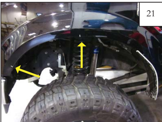
Install Clip (CL1-0022) in two locations. See Step 22 & 23.
