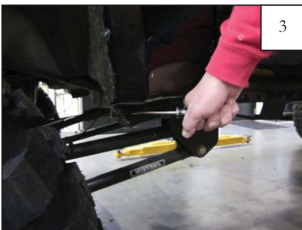
Using a pry tool, remove factory installed tufloc rivet located at the bottom rear of the wheel well.
