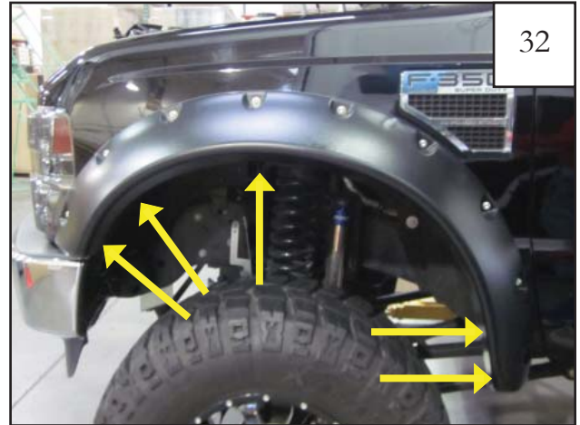
Install flare using screw (SW1-0056) through holes indicated.
