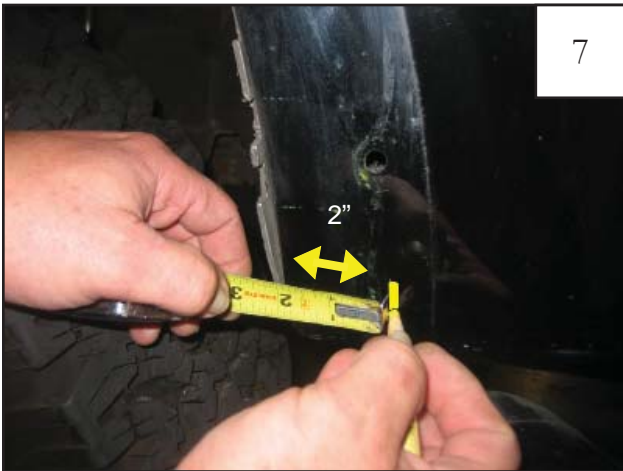
Using a tape measure and a grease pencil, mark a line 2" toward door seam from fender lip (at bottom edge).
