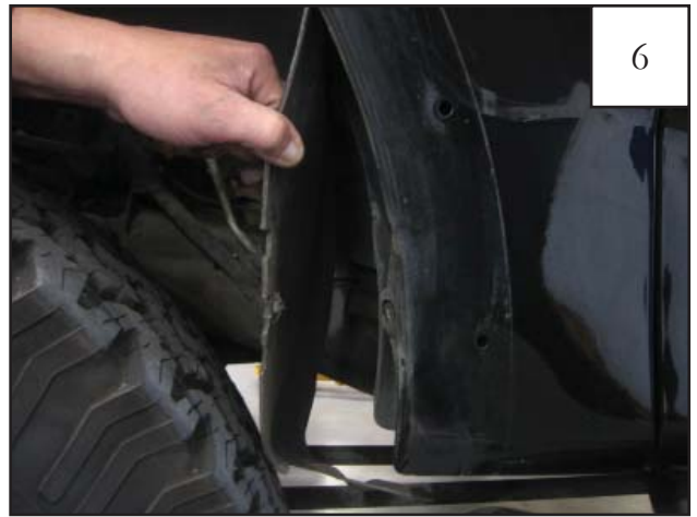
Pry splash shield loose from rear of wheel well area. There are a few factory clips that will pop.
