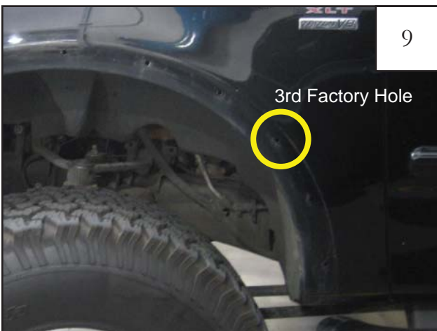
Third factory hole location. If the truck did not come with factory flares and there are no factory holes on fender, refer to Step 10.
