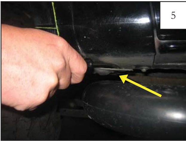
Use a trim tool to remove one plastic fastener located at bottom rear of splash shield (next to bottom of door seam).
