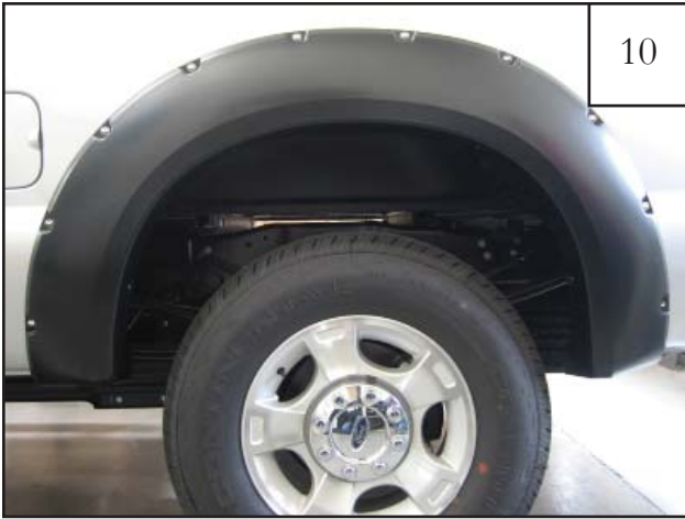
Completed rear flare installation.
