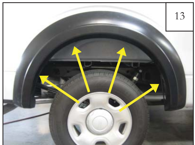
Hold flare to vehicle and mark the location with a grease pencil of the four holes in the flare. Note: Rear flares are similar enough that either will fit against the body of both sides. The wheel well hole locations will be wrong if the flare is on the wrong side. Driver's side flare is marked with an "L" and passenger's side flare is marked with an "R".
