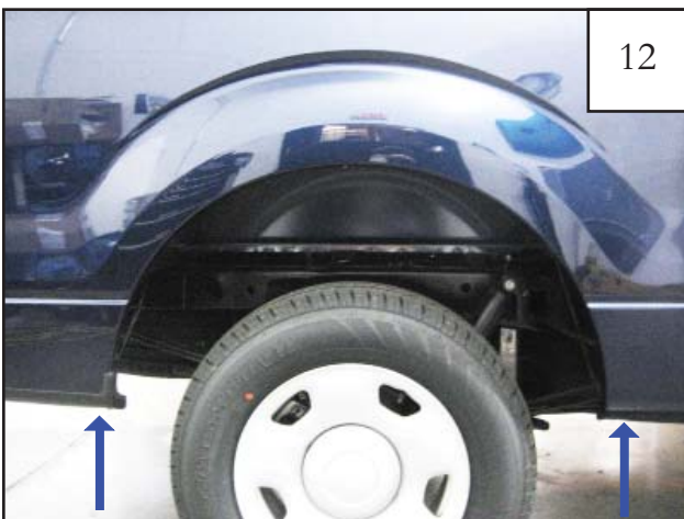
Remove two factory bolts with a 10mm socket wrench. (Note: New hardware is being supplied see Step 17)
