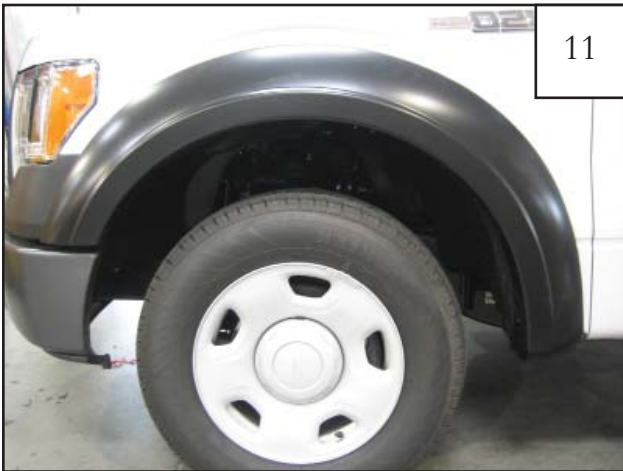
Completed front flare installation.
