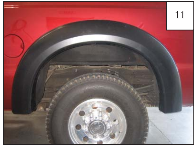
Completed rear flare installation.
