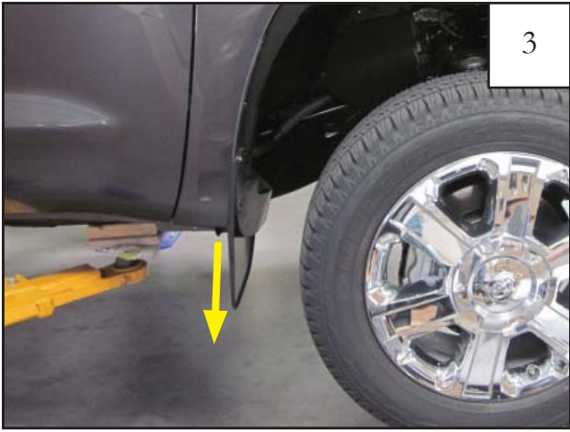
3 Remove push retainer from underside of factory mud guard.
