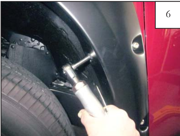
Start supplied Screw (SW1-0036) through top rear hole in flare and into factory hole in rear of wheel well. Do not tighten.
