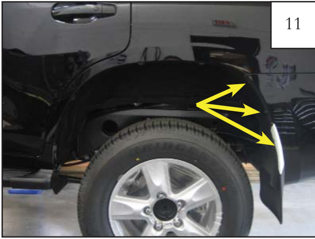
Using a socket with a T30 Torx bit, remove three factory screws. Discard.
