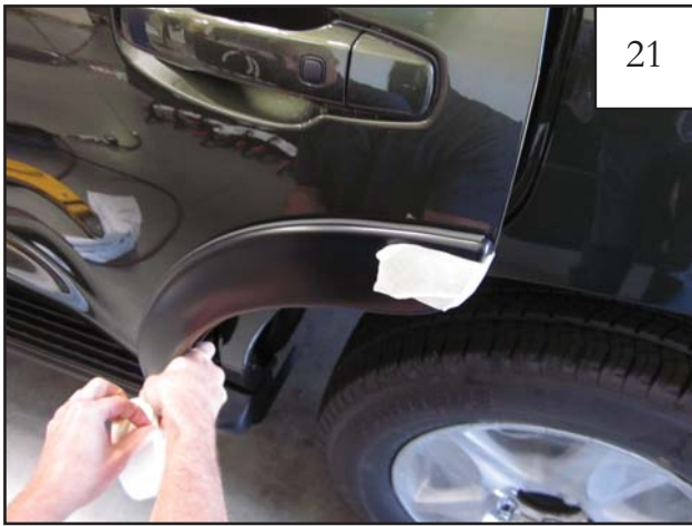
Position Door Piece (without edge trim) on door. Line up with the top and bottom of door edge. Use masking tape to hold flare in place.
