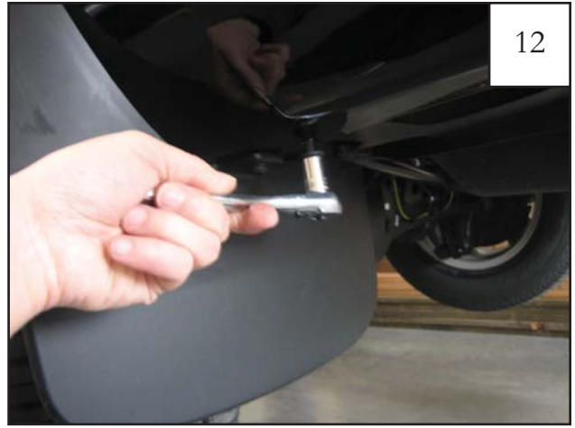
Using a 10mm socket, remove one factory bolt from underside of bumper at mud flap area. Discard.
