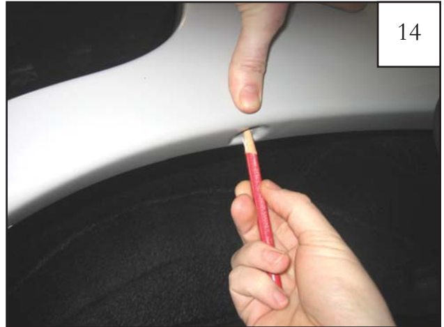
Using a grease pencil, mark four clip locations on fender of flare, using holes in flare as a guide. Remove screws and remove flare from fender.
