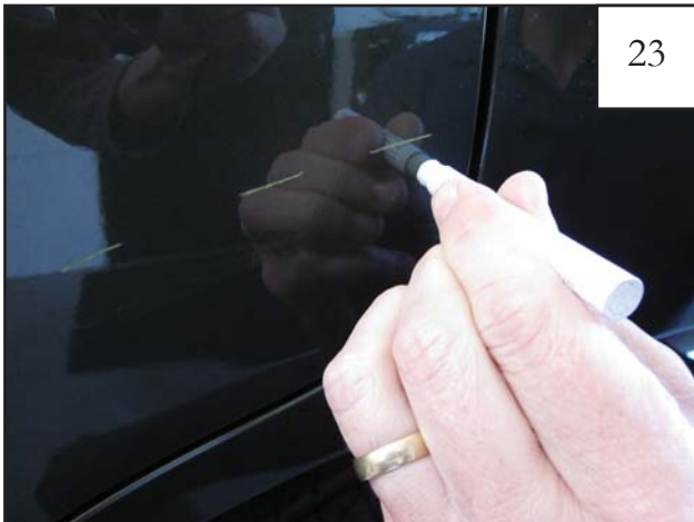
Using Primer Ampoule, apply primer to door \frac{1}{4} " below the line marked with grease pencil. NOTE: Allow primer to dry for five (5) minutes before continuing installation.
