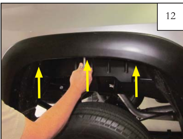
Hold the flare firmly on the fender. Start three supplied 20mm Hex Screws (SW1-0036) through the top center holes of the flare and into factory holes in fender.
