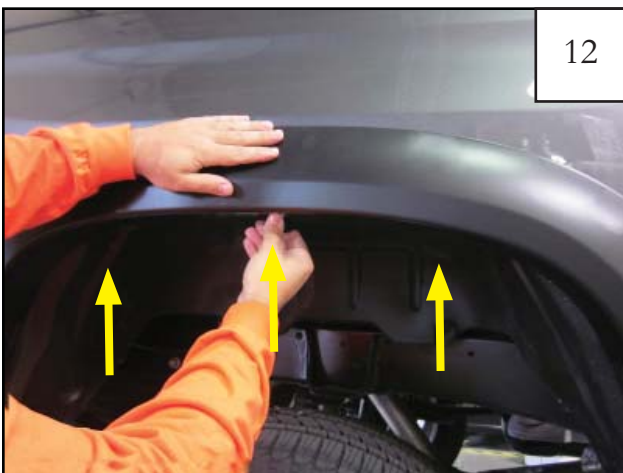
12 Hold the flare firmly on the fender. Start three supplied 20mm Hex Screws (SW1-0036) through the top center holes of the flare and into factory holes in fender.
