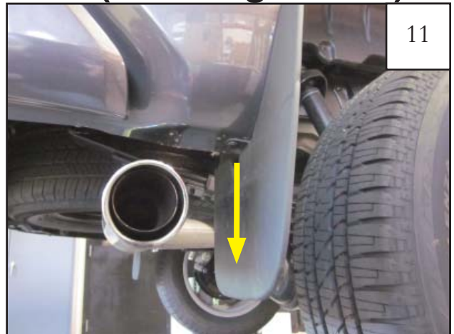
11 Remove factory push retainer from underside of factory mud guard and remove mud flap.
