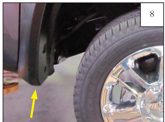
8 Install supplied push retainer (RV1-P009) into factory hole on underside of mudguard.
