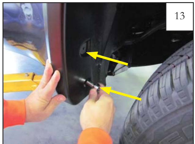
13 Start two supplied 20mm Hex Screws through the rearward most holes of flare and into the factory hole in fender.
