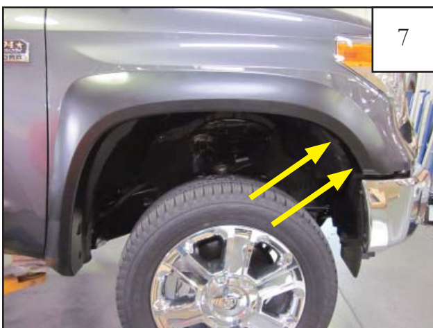
7 Start two supplied 20mm Hex Screws through forward most holes in flare and into factory hole locations.
