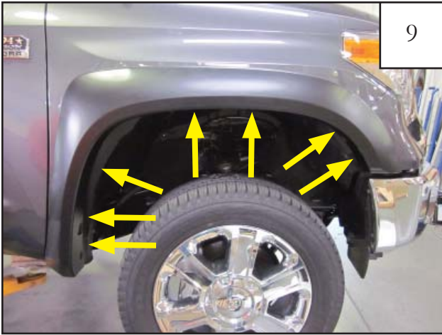
9 Ensure flare is properly positioned and tighten all screws. (Repeat for other side of vehicle) Installation Complete.
