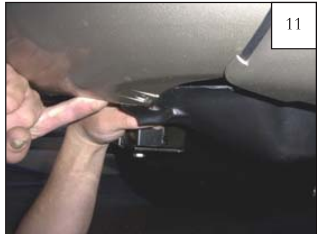
Pull down bumper cover and splash shield.
