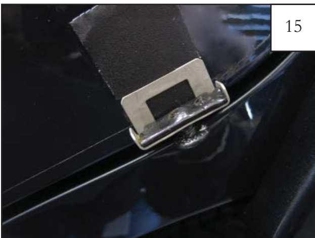
Hand start serrated-flange screws through each clip. The end of the shaft should be flush with the uppermost edge of the clip.
