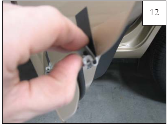
Install the clip over the black tabs installed in step 10.
