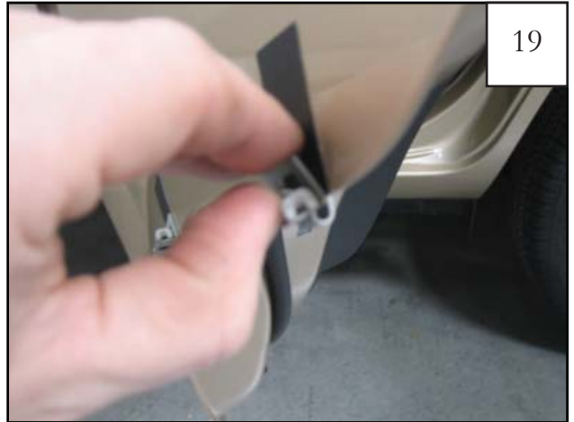
Install the clip over the black tabs installed in step 17.
