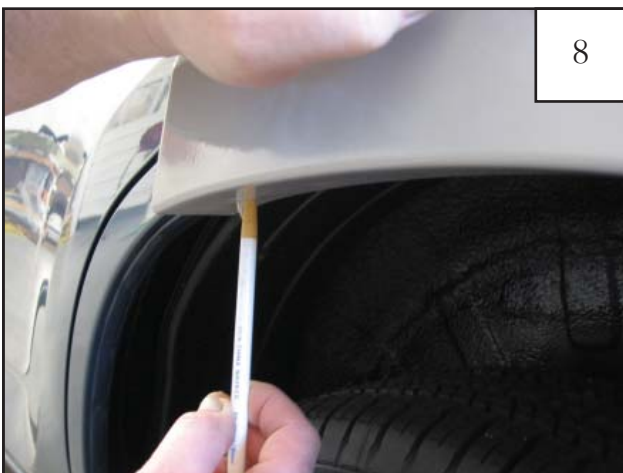
Hold the flare firmly on the fender. Using holes in flare as a guide, mark four clip locations with a grease pencil.
