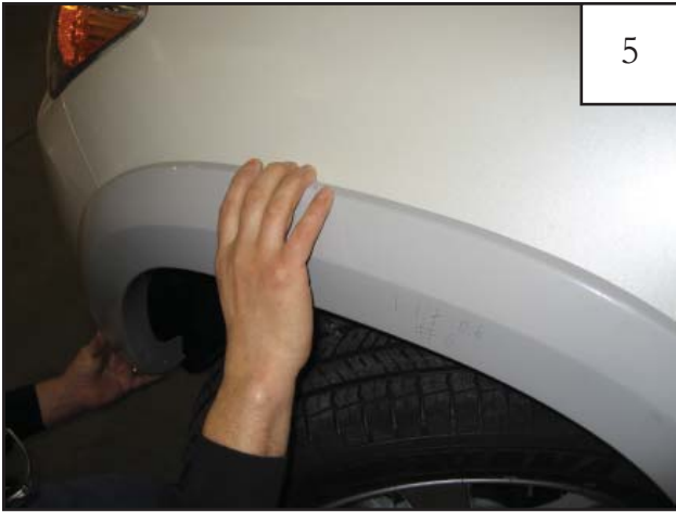
Replace flare on fender, aligning holes with the holes in clips.
