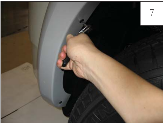
Start supplied serrated-flange screws through the three forward holes in flare and into the "S" clips installed in step 4. Using a right angle or stubby Phillips #2 screwdriver, tighten all screws.
