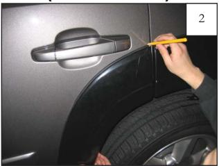
Position Door Piece correctly on door. Using a grease pencil, trace outline of flare on door.
