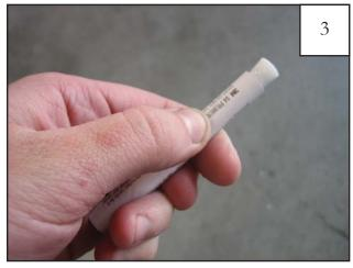
Open door. Break supplied Adhesion Primer Ampoule to allow primer to saturate applicator tip.
