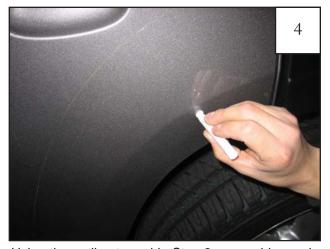
Using the outline traced in Step 2 as a guide, apply primer to door in areas that tape pads will contact (about two ampoules will be needed per side). WARNING: DO NOT APPLY PRIMER ABOVE AREA TO BE TAPED!
