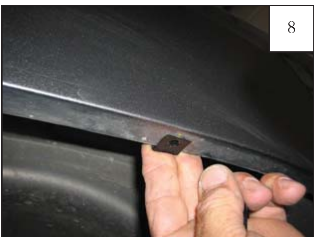
Center a supplied Clip (NU1-0007) over the upper two marks made in Step 6. Clips may need to be adjusted to align with holes in flare. Note: The raised collar on the Clip should face upward into the interior of the fender.
