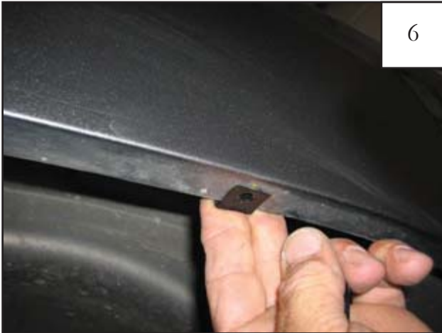
Center a supplied Clip (NU1-0007) over the upper two marks made in Step 4. Clips may need to be adjusted to align with holes in flare. Note: The raised collar on the Clip should face upward into the interior of the fender.
