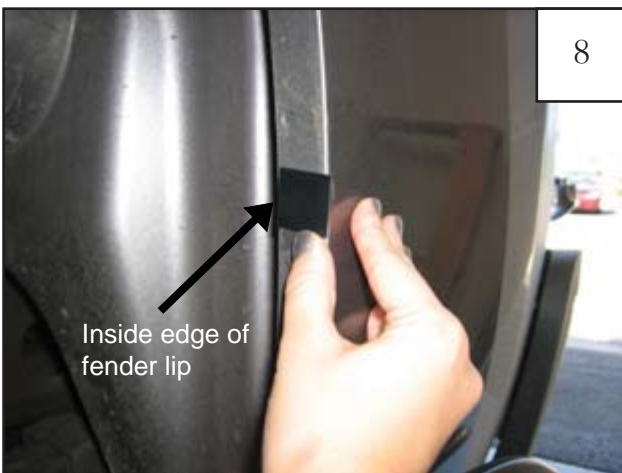
Center a supplied Tab (MT1-0002) over the six remaining marks made in Step 4, aligning edge of Tab with inside edge of fender lip (Tab may extend over outside of fender).
