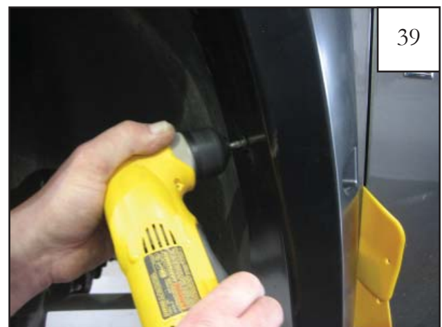
Install Screw (SW1-0056) through flare and into hole in sheet metal in both locations.
