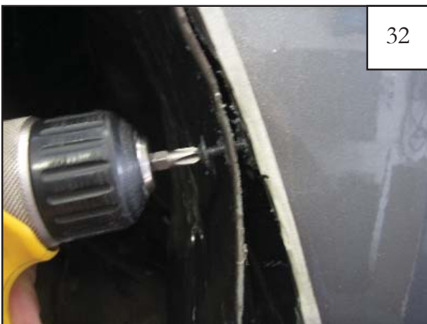
32 Starting with the top location, fasten inner fender metal to bent tabs of outer fender with Screw (SW1-0056)s through holes drilled in last step (3 locations).
