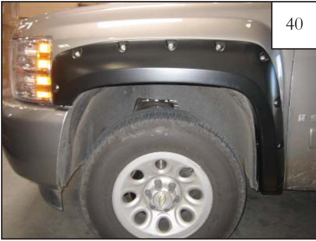
Reinstall wheel. Completed front flare installation.
