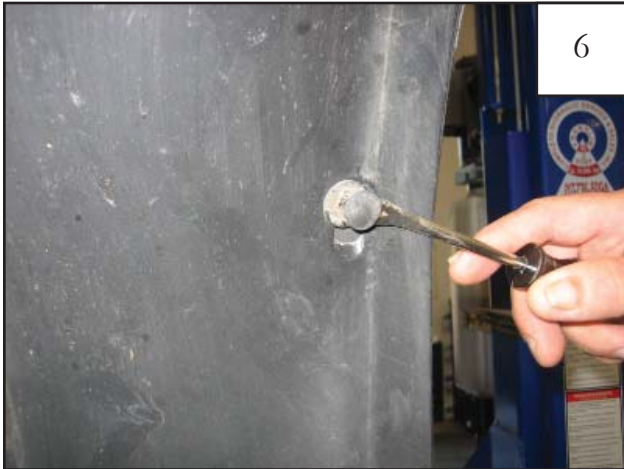
Using a pry tool, remove plastic factory fastener from wheel well liner located above the two factory screw locations.
