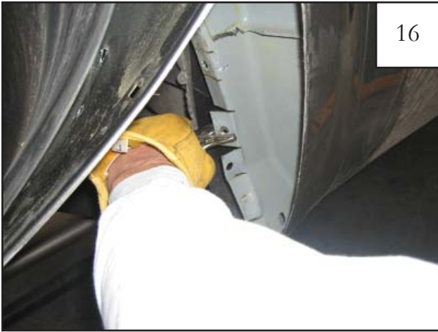
Bend lip straight with pliers between cuts made in previous step. NOTE: In Step 20, existing cuts will be extended after reference lines are marked.
