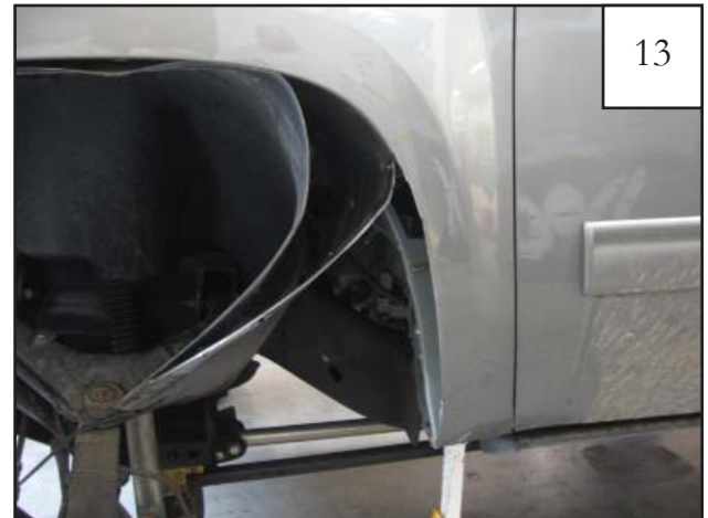
Bend inner fender metal away from fender.
