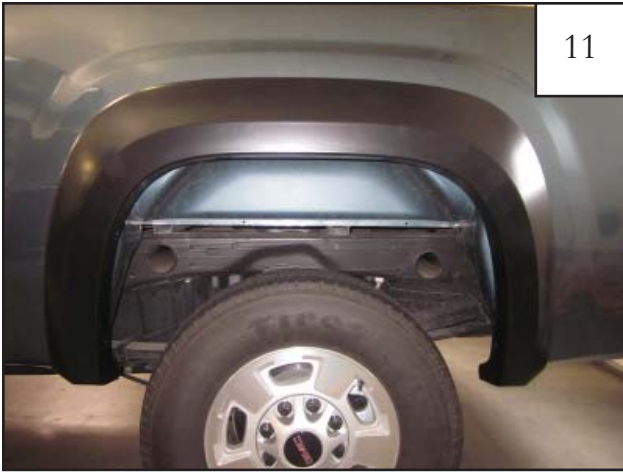
Completed rear flare installation.
