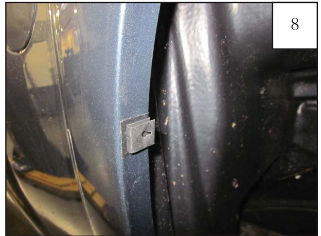
Slide a supplied Clip (CL1-0005) over each Tab. Clips may need to be adjusted to align with holes in flare.
