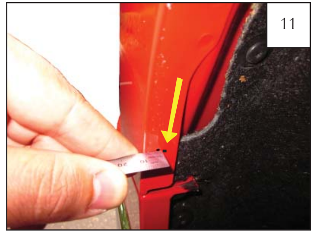
Remove the flare. At the marked locations made in Step 9, measure inward 22mm from the edge of the fender. These are the marks to be drilled. Note: Marks at 22mm may be on either side of the marks made in Step 9..
