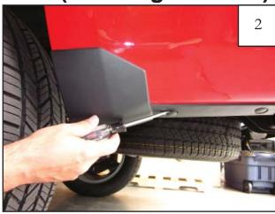
Using a pry tool, remove factory retainers in bottom of factory rear mudguard. Remove mudguard and discard.
