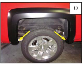
Re-install supplied screws (SW1-0056) into two lower most holes.
