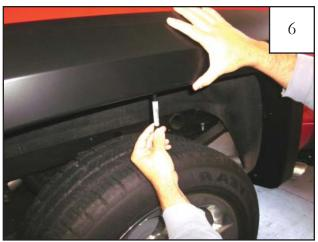
Using a grease pencil, mark five locations using the holes in the flare as a guide.
