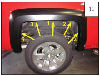
Install supplied self-tapping screws (SW1-0066) into pilot holes in the order indicated. *PRESS FLARE TOWARD VEHICLE AND TIGHTEN ALL SCREWS*
