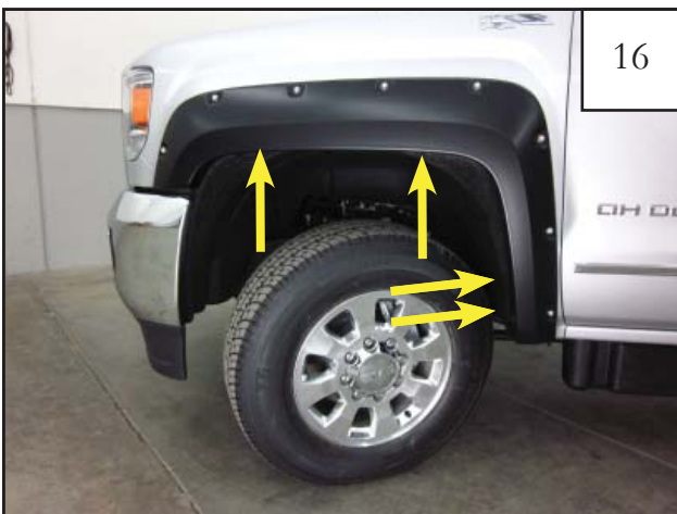
While holding Flare on vehicle, install supplied screw (SW1-0056) into the two upper and lower factory holes locations. Do not fully tighten at this time.
