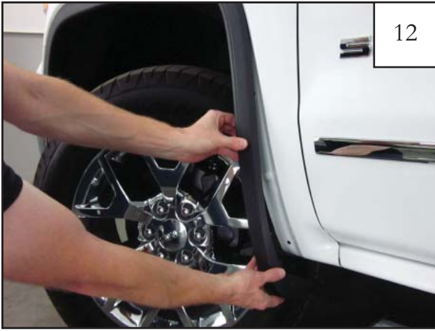
Starting at the lower rear end of the factory flare, firmly grip part and pull to remove from vehicle. Note: You will hear popping sounds as the factory fasteners release from vehicle. This is normal.
