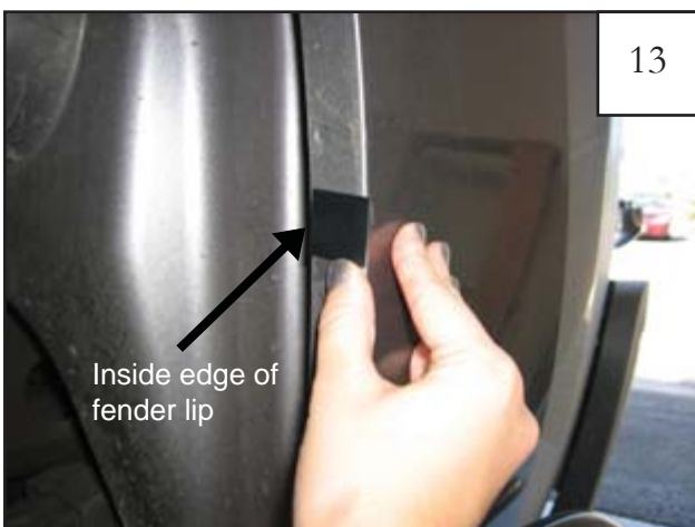
Center a supplied Tab (MT1-0002) over the six remaining marks made in Step 9, aligning edge of Tab with inside edge of fender lip (Tab may extend over outside of fender).
