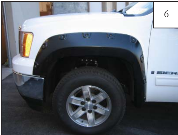
Completed front flare installation.
