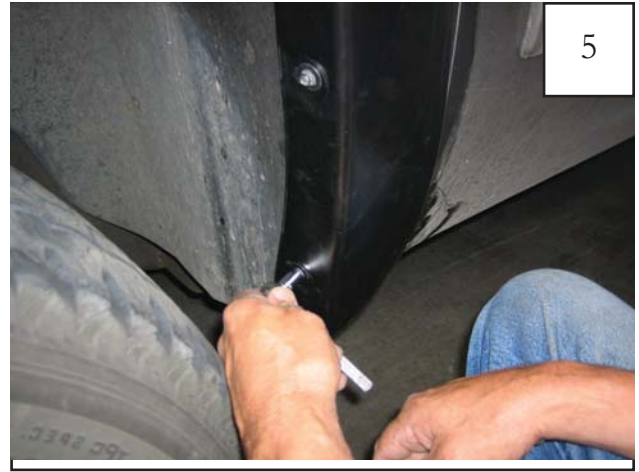
Position flare on fender and reinstall six factory screws removed in Step 4. If needed, use an awl to locate holes.
