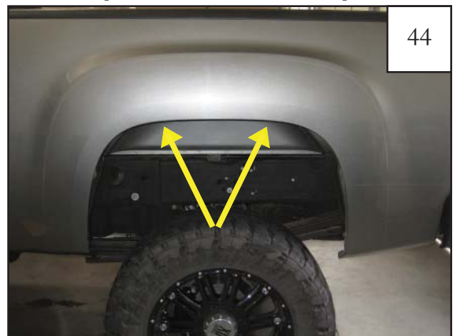
Tufloc locations NOTE: If fender liner is installed. Remove factory tuflocs.
