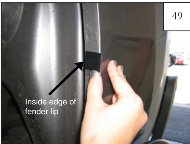
Center a supplied Tab (MT1-0002) over the six remaining marks made in Step 46, aligning edge of tab with inside edge of fender lip (tab may extend over outside of fender).
