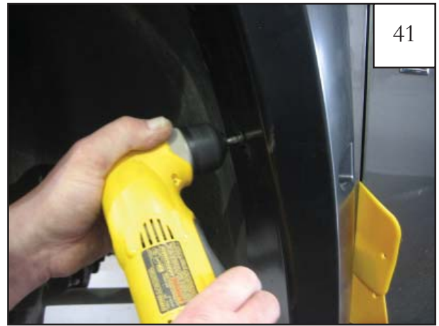
Install Screws (SW1-0056) through flare and into hole in sheet metal in both locations.
