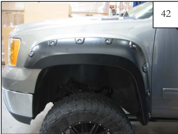
Reinstall wheel. Completed front flare installation.
