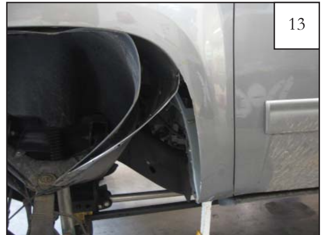
Bend inner fender metal away from fender.
