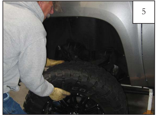
Support vehicle and remove tire.
