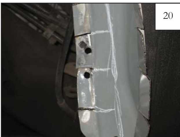
20 Using outer edge as a guide mark along flange parallel with the inner wall. Mark flange to extend cut lines to line parallel with the inner wall.
