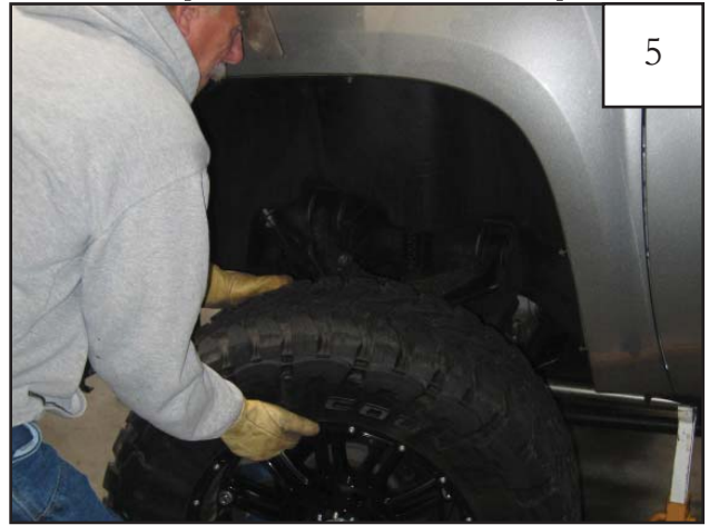
Support vehicle and remove tire.
