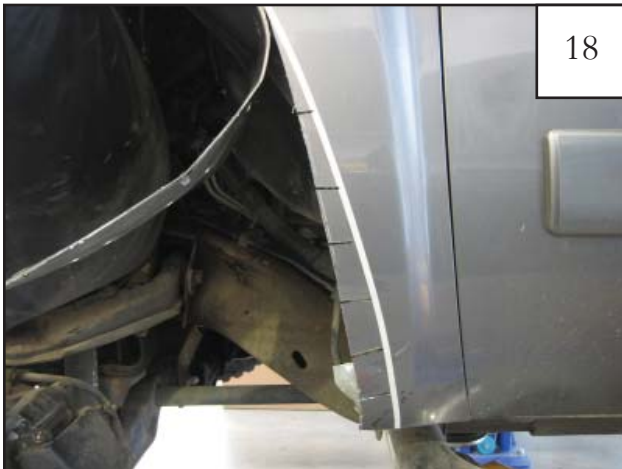
18 Cut fender approximately every 2" up to edge of masking tape.
