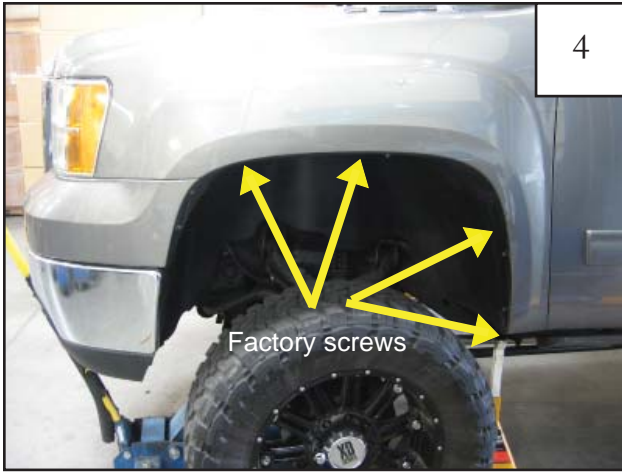
Using a 7mm socket, remove four factory screws from wheel well and save for reinstallation.
