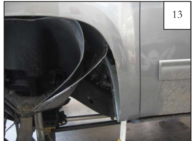
Bend inner fender metal away from fender.
