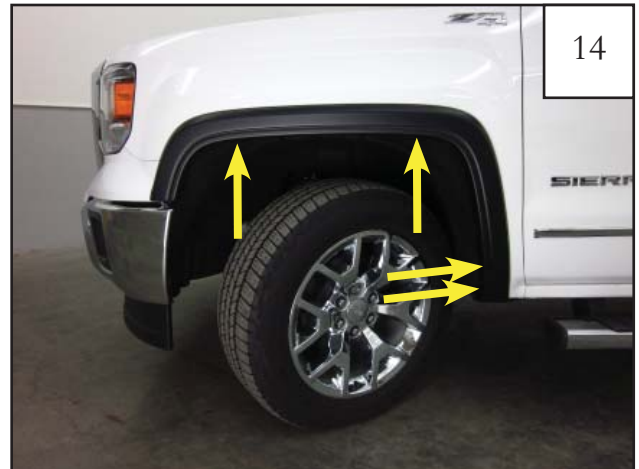
14 While holding Flare on vehicle, install supplied screws (SW1-0056) into the two upper and lower factory holes locations. Do not fully tighten at this time.
