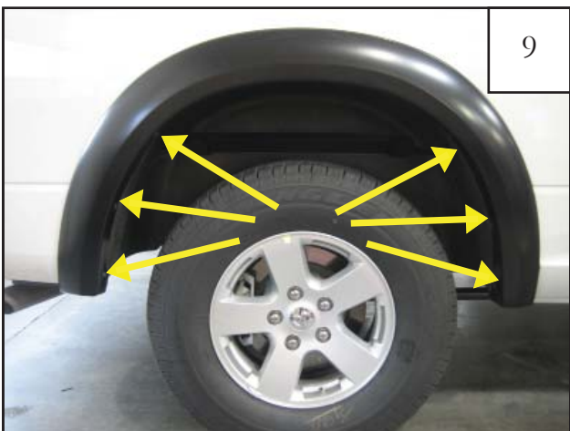
Hold flare in place while you start six additional supplied screws using a Phillips Head Screwdriver. Do not tighten.
