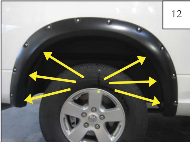
Hold flare in place while you start six supplied screws (SW1-0056) using a Phillips Head Screwdriver. Do not tighten.
