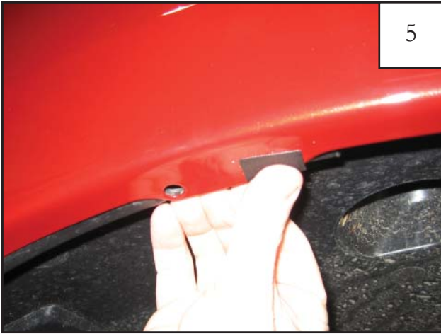
Install 1"x1.5" Black Tab over existing factory hole. There are two holes at the top center location. Refer to step 4 for proper hole for installation.
