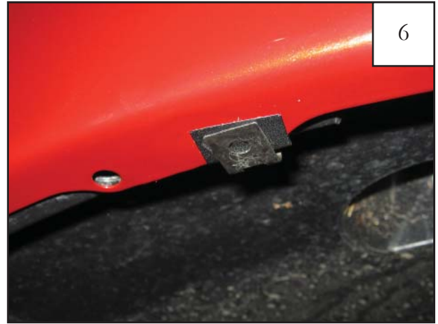
Install #10 U-Clip over 1"x1.5" Black Tab.
