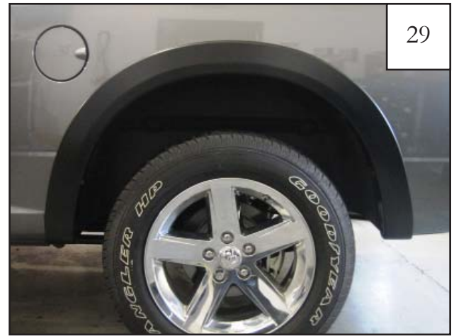
Completed rear flare installation.
