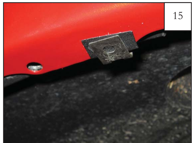
Install #10 U-Clip over 1"x1.5" Black Tab.
