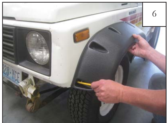
Hold front flare in position on fender and, using a grease pencil, mark each hole location on sheet metal.
