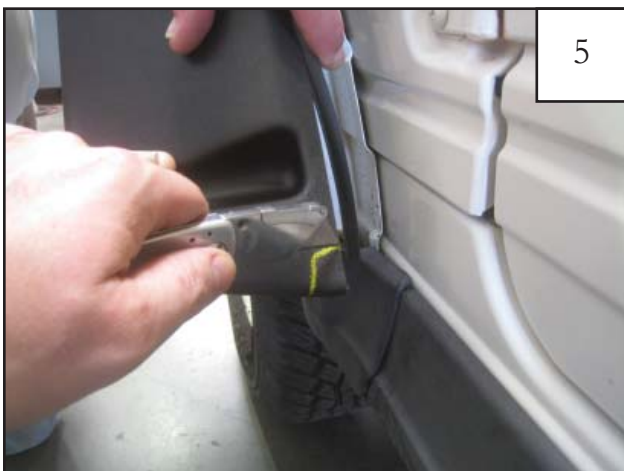
Optional Step in Cases Where Factory Rocker Moldings are Still on Vehicle: Hold flare in position on vehicle and mark where it interferes with rocker molding. Cut a notch into the flare on mark with utility knife.
