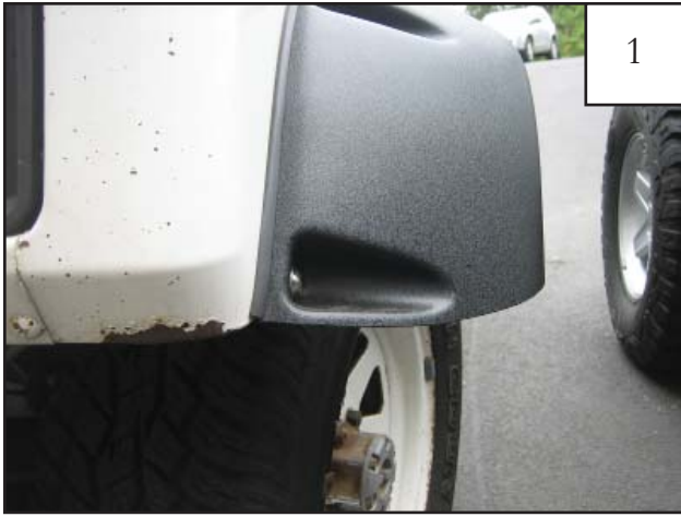
The front and rear flares are similar in shape and size. Front flares are labeled on the inside with 60015-07 and rears are 60016-07. Pictured above is the front flare.
