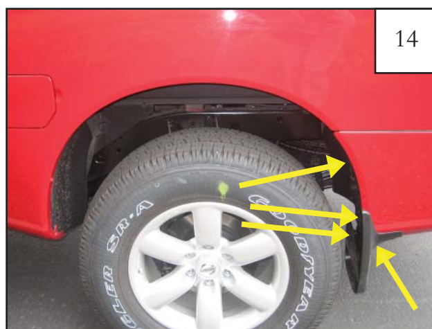
Driver Side Flare: Remove factory mud flaps if installed, and one extra unpainted screw above mud flap.
