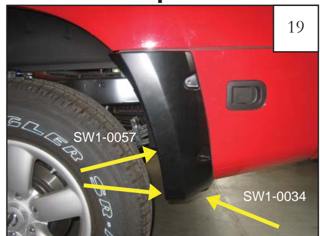
Hold the door piece flare up to the door and line up the holes in the flare with the three factory holes. Start the Screw (SW1-0034) into the bottom grommet first, then move onto the Screw (SW1-0057). Do not fully tighten screws.
