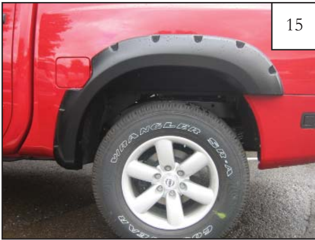
Driver Side Flare: Hold (LR) flare in position on fender with moderate pressure. Ensure the notch in the flare is positioned correctly with the gas door.
