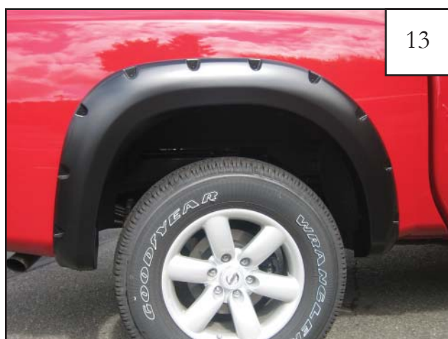
Passenger Side Flare: Completed rear flare installation.
