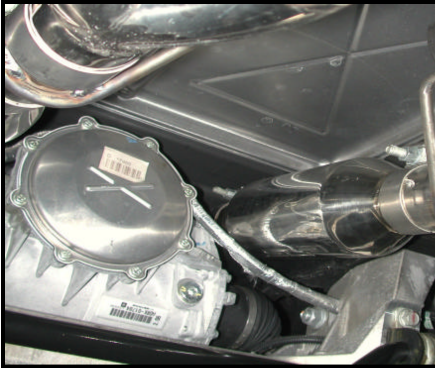
Photo 5: Resonators/Mufflers Installed on Over-axle Pipes
